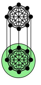
In regular graphs  $\frac{e(S,V-S)}{\min\{vol(S),vol(V-S)\}}$  is equivalent to  $\phi(S) = \frac{e(S,V-S)}{vol(S)}$  assuming  $S \leq \frac{n}{2}$
