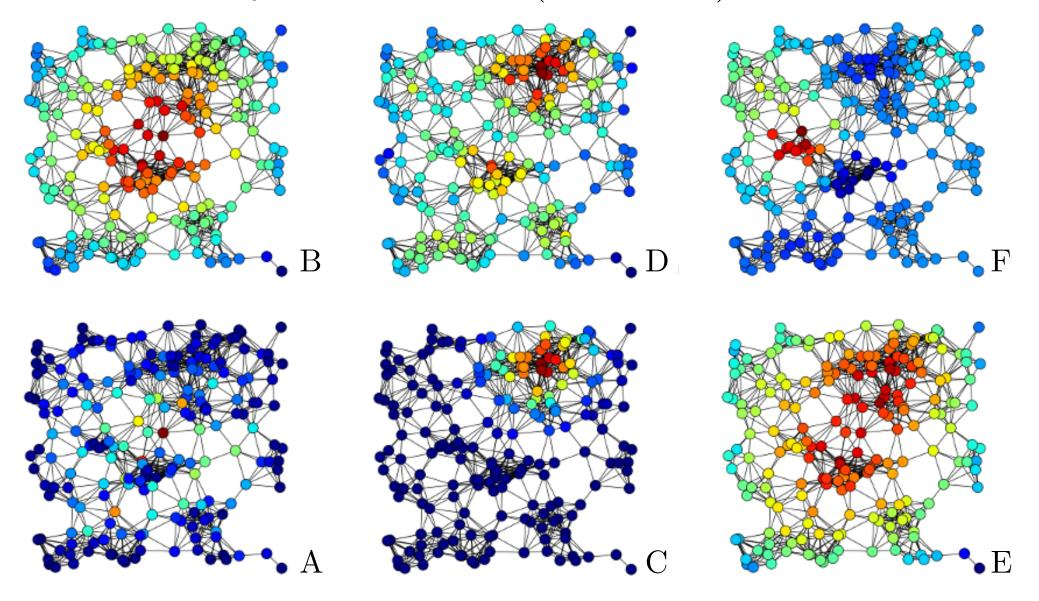
Examples of A) Betweenness centrality, B) Closeness centrality, C) Eigenvector centrality, D) Degree centrality, E) Harmonic Centrality and F) Katz centrality of the same graph\*.
